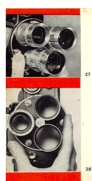
locking catch, thus freeing it (27). To swivel the turret (either clockwise or antichlockwise), use the three knobs fitted between the lenses, to avoid any risk of modifying their settings. Once the catch has clicked into place, the lens chosen for filming is properly aligned (upper position) (28).
