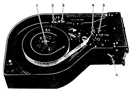
Fig. 13-12. Eclair NPR magazine (feed side). Courtesy of Eclair International Diffusion.
