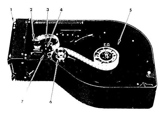
Fig. 13-13. Eclair NPR magazine (take-up side). Courtesy of Eclair International Diffusion.
